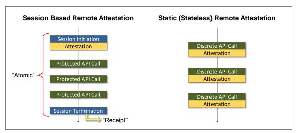
The state diagrams below illustrate the instruction flow from the RPS to the TEE:
